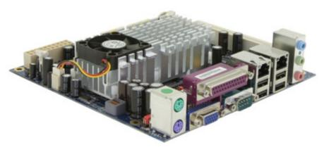
The VIA EPIA EK Mini-ITX mainboard is available with the 1GHz or fanless 800MHz VIA Luke CoreFusion<sup>™</sup> processor platform and boasts a rich array of connectivity and digital media features to make possible a new generation of bandwidth efficient network devices focused on digital media applications.
